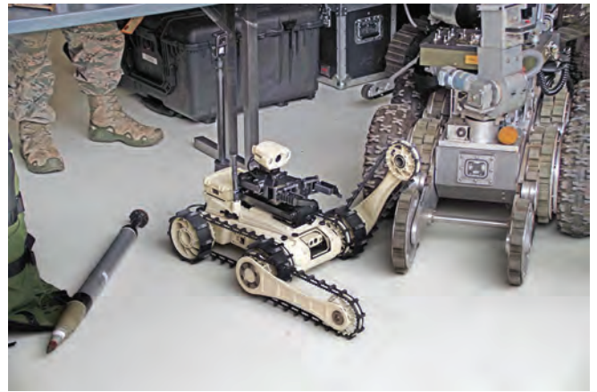
Lightweight robot used for assessing IEDs (Improvised Explosive Devices) in the field. Photo Gerald Tompsett
